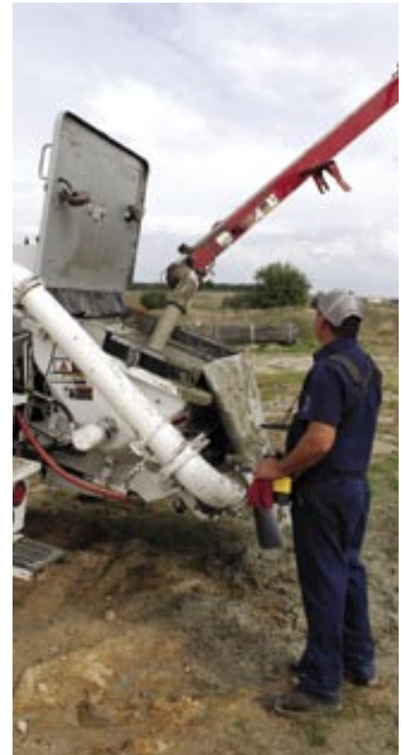
Pump to pump operation is monitored using Schwing's Vector Control System which provides valuable two-way communication between pump and operator.
