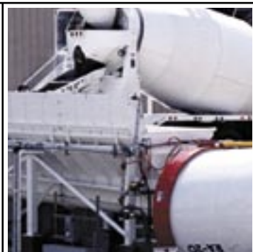
Screw troughs (backup or drive over) allow drivers to dump up to 10 yards of leftover concrete at once for gradual feeding to the RA-20.
